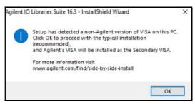
Important: <u>Must</u> be installed as **Secondary** VISA Make sure NIVXI1600 is installed first
