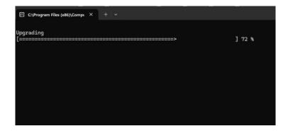
After the tool has applied the update file, the mainframe will reboot. Be aware that additional update steps are executed during the reboot phase. For example, if the FPGAs on the ALI cards require an update, the boot process could take 10 or 15 minutes.
